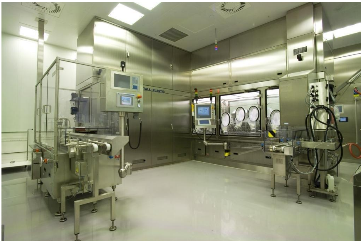
Figure 1. Filling line in a pharmaceutical facility. Tubs are placed on the conveyor to the left, passed through the e-beam isolator in the middle to the filling area to the right.
