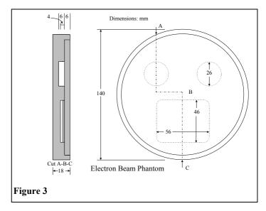
of 3 mm pellets enclosed in disc holders 25 mm diameter, 6 mm thickness) and film routine dosimeters. If used without the 6 mm thick top plate, this design is also suitable for use at energies down to 4 MeV.
