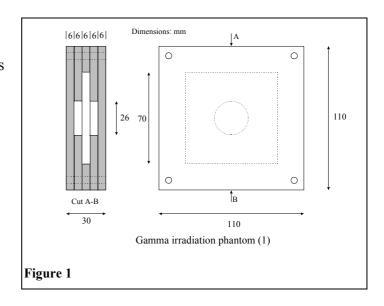
This geometry is suitable for either dichromate or ceric-cerous dosimeter ampoules, or alanine pellets in cylindrical holders. The orientation of the phantom with respect to the source is important and must be such that direct radiation from the source passes through the shortest axis of the phantom.
