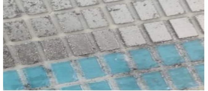
Fig. 3. Ferromagnetic foil after the milling process. The foil is fixed to a PMMA substrate (white) using electrostatic tape (blue) which allows the foil to be diced in a controlled way.
