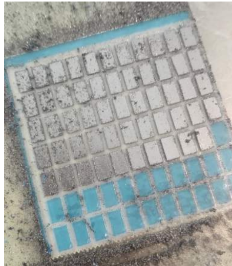
Figure 6.12: Ferromagnetic foil after being milled. The blue spots correspond to the blue tape that serves as interface between the PMMA (white) surface and the foil. Some foil pieces have fallen off from the blue tape while milling. The other pieces are easily peeled away by dipping them in an acetone bath.
