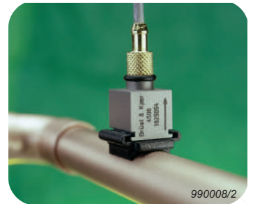
Fig. 6 Mounting Clip with Thick Base UA-1475 can be filed down to suit the needs of your mounting surface. Here it is mounted on a tube with Type 4508
