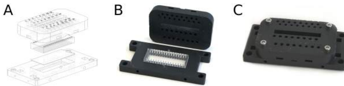
Figure 5.5: A) Sketch of the 3D printed clamp with the MDA glass substrate and PDMS lid. B) 3D printed, magnetically clamped microfluidic interface. C) Magnetically clamped microfluidic interface including four bolts for added compression.
